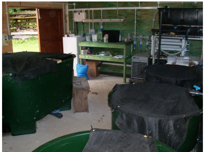
Fig.20. Recirculation system for maternal incubation
